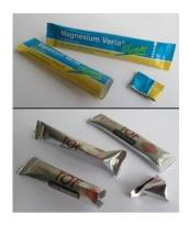
The Laser Perforation Opening Aid, currently used by Verla-Pharm Arzneimittel for Magnesium Verla, can be opened quickly and simply and is clearly marked by arrows at one end of the stick. Traditionally the aperture for conventional 'notch' openings is approximately 50 per cent of the width. Using the PET/Alu/PE-LD easy-tear laminate and laserperforation allows 100 per cent of the aperture to be opened.
