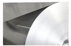
Constantia Flexibles: Aluminium foil < 5µm
