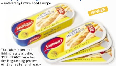
opening of rectangular fish cans. By combining the flexibility and strength of the extrusion coated 70 µm foil, a tabbed lid provides both full protection for the autoclave sterilised product and easy peelability for opening. For the consumer, the new alufoil lid system eliminates the difficulties and hazards of the ring-pull system previously widely used. For the packer, the beaded lid performs without difficulty on the established canning lines.
